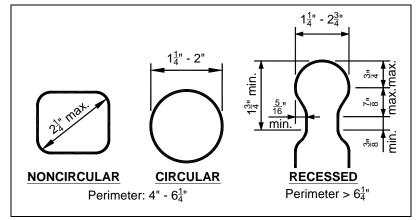
FIGURE 37: HANDRAIL GRASPABILITY TYPES/GEOMETRY
