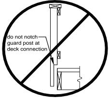
FIGURE 28: NOTCHING AT GUARD POSTS
