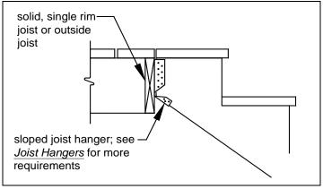
FIGURE 34: STAIR STRINGER ATTACHMENT DETAIL
