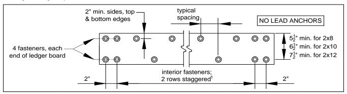
FIGURE 20: LEDGER BOARD FASTENER SPACING AND CLEARANCES
