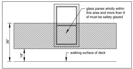
FIGURE 41: SAFETY GLAZING AREA AT WALKING SURFACE
