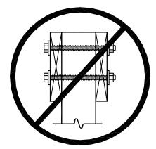
FIGURE 10: PROHIBITED POST-TO-BEAM ATTACHMENT
