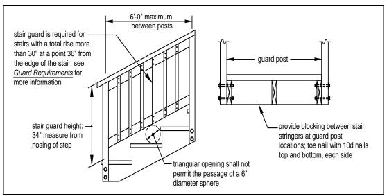
FIGURE 36: STAIR GUARD REQUIREMENTS
