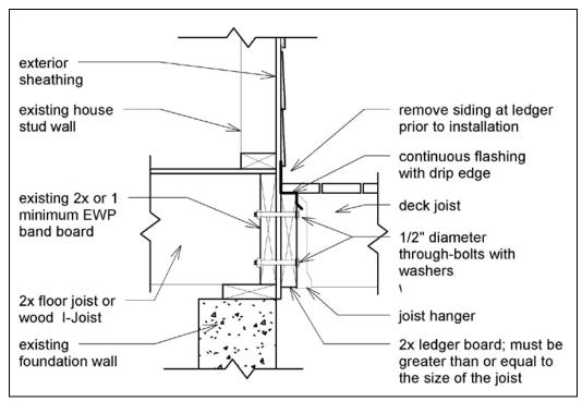
FIGURE 14: ATTACHMENT OF LEDGER BOARD-TO-BAND BOARD
