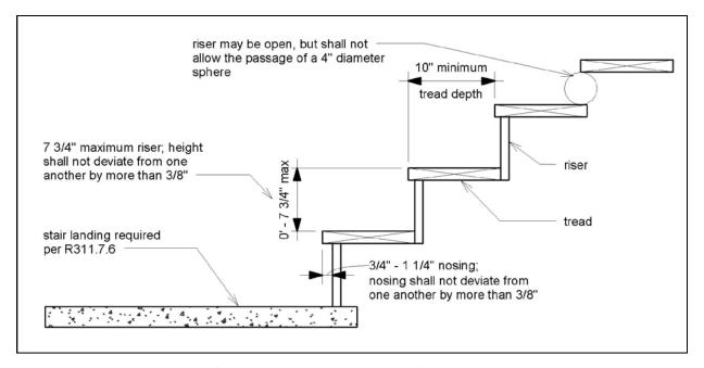
FIGURE 32: TREAD AND RISER DETAIL
