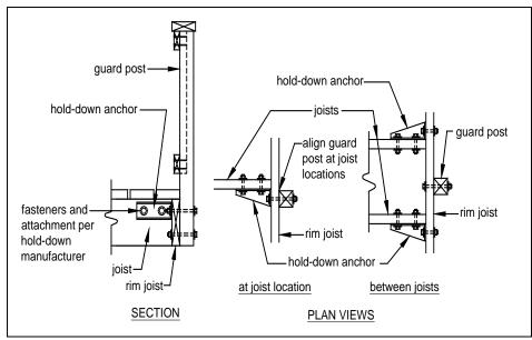
FIGURE 31: GUARD POST-TO-RIM JOIST DETAIL
