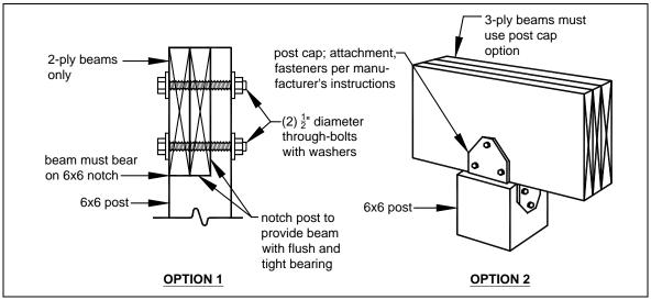
FIGURE 11: POST-TO-BEAM CONNECTION OPTIONS
