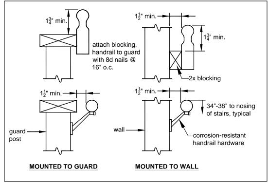
FIGURE 38: HANDRAIL REQUIREMENTS
