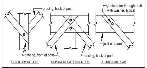
FIGURE 24: TYPICAL CONNECTIONS OF DIAGONAL MEMBERS
