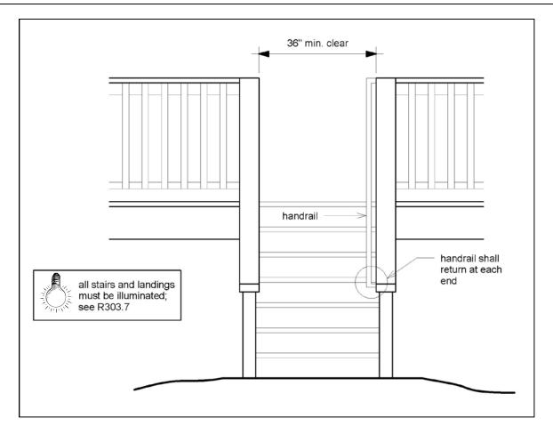
FIGURE 39: MISCELLANEOUS STAIR REQUIREMENTS
