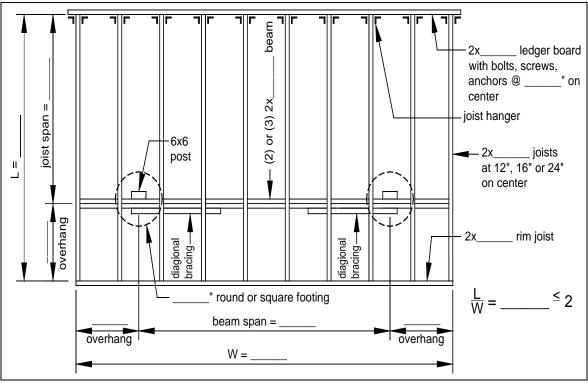
FIGURE 7: TYPICAL DECK FRAMING PLAN
