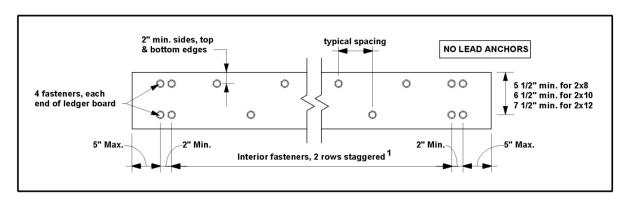
FIGURE 20: LEDGER BOARD FASTENER SPACING AND CLEARANCES
