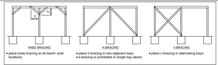
FIGURE 22: DIAGONAL BRACING AT BEAM-POST LOCATIONS (all decks)
