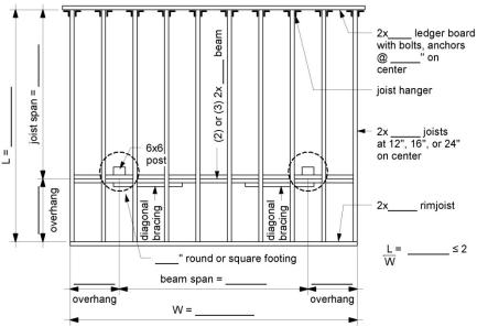
FIGURE 7: TYPICAL DECK FRAMING PLAN
