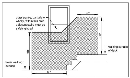
FIGURE 42: SAFETY GLAZING AREA AT STAIRS
