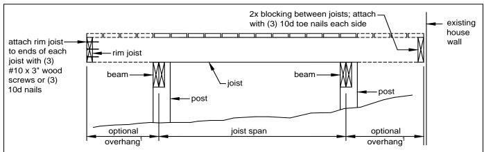
FIGURE 4: JOIST SPAN - FREE-STANDING DECK<sup>2</sup>
