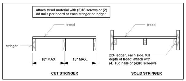
FIGURE 35: TREAD CONNECTION REQUIREMENTS
