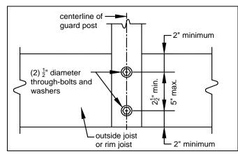
FIGURE 29: GUARD POST ATTACHMENT DETAIL
