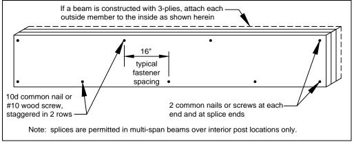
FIGURE 6: BEAM ASSEMBLY DETAIL
