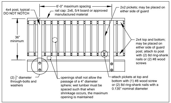
FIGURE 27: TYPICAL GUARD DETAIL
